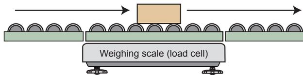
When HPDF is used, as the effects of vibration are eliminated, the peak value can be taken as the weight of the measured object.
