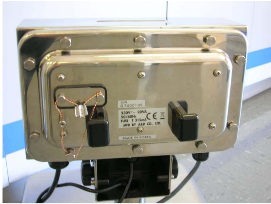
Figure 2 Calibration switch sealing
