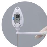
Temperature can be measured with the sensor mounted in a sheath holder hole
