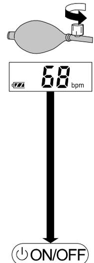
Note: Model UM-101 has an automatic power-off function.
