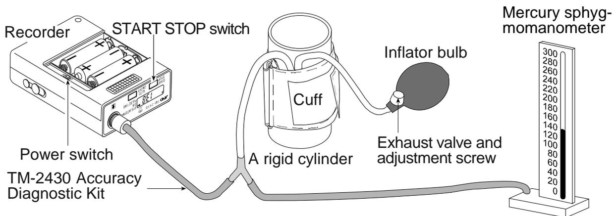
**Step 3** Keep the pressure at the air socket to atmospheric pressure.
