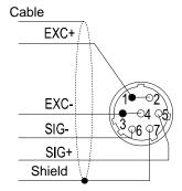
Connection available for a cable shorter than 5 m. (Recommended wire cross-sectional area: 0.5 mm<sup>2</sup> or greater)
