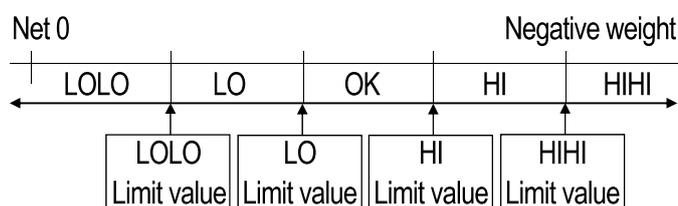
Note: To start the take-away check weighing, be sure to use the TARE switch to tare the weight of the container filled with objects. The ZERO switch may zero the display, and the scale goes below the zero point by taking out the objects. Then, the auto-tare function does not work.
