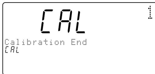
6. Press the **CAL** switch and re-attach the calibration switch cover.
