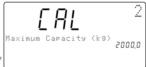
5. Press the **ENTER** key again to store the capacity entered and the remote scale is ready to be calibrated.
