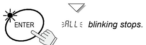
3. Press the **ENTER** key again to clear all of ID memories. Press the **RESET** to exit without clearing ID memories. The display will return to normal.
