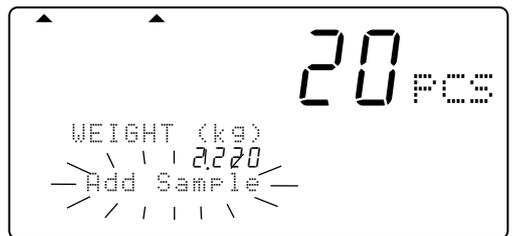
5. Press the **ENTER** key. The display will show "-----" for a moment while calculating the unit weight. After a moment the display will show the count, total weight and unit weight.
