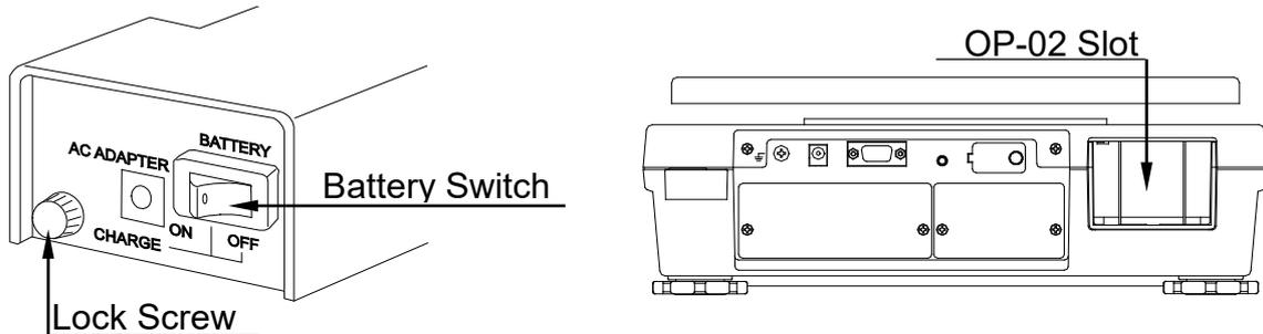
2. Tighten the lock screw on the battery pack.
