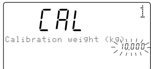
⚠ If you know the exact weight value, or if you wish to use a different weight, use the **0** → **9** and **.** 10-key pad to display the desired calibration weight. (For example: Using 10kg calibration weight that actually weighs 10.002kg.)
