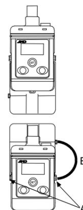
When the AD-8527 is in use, the cap can be attached on the bottom.
