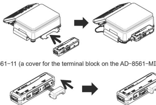
(7) AD8561-11 (a cover for the terminal block on the AD-8561-MI04)
