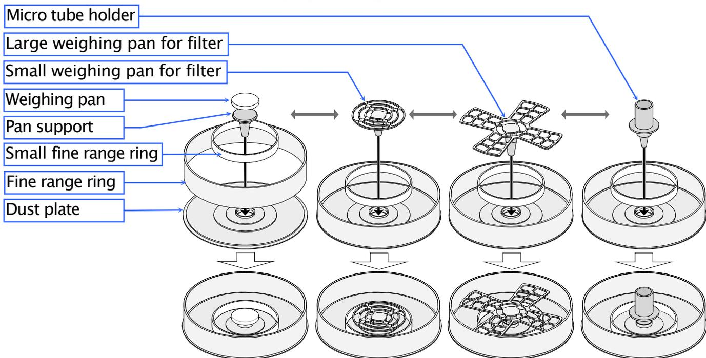
Choose the weighing pan appropriate to the filter size.
