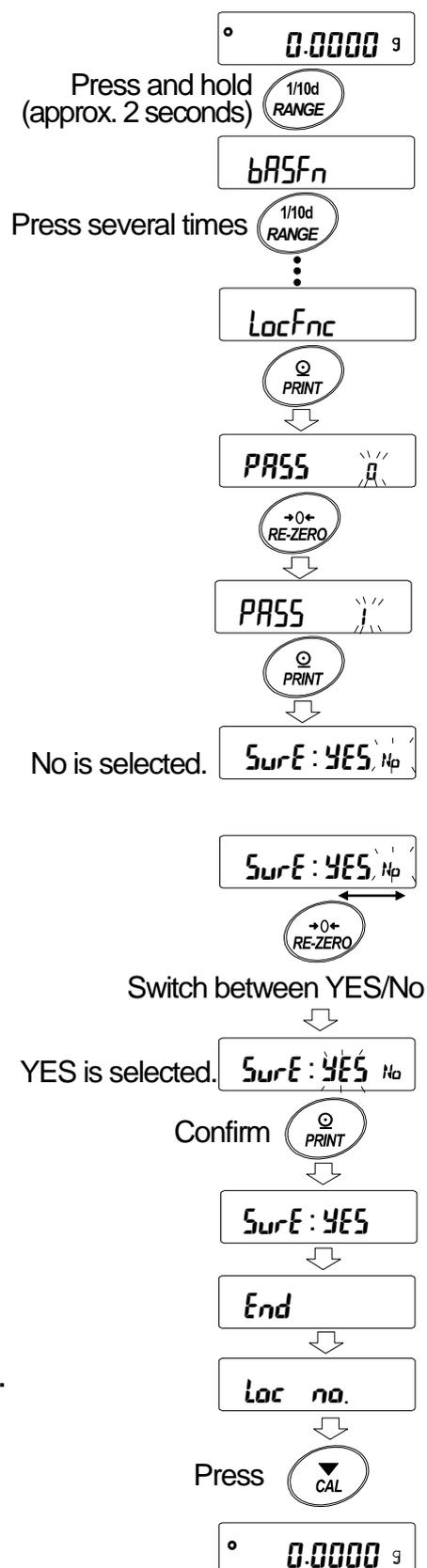
**Note** When the balance software version is 1.50 to 1.64, only “Not used (0)” or “Used (1)” is available.
