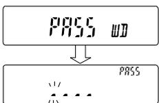
This is the display to prompt you to enter a password. When the password function is used, the correct password must be entered for the balance to enter the weighing mode.
