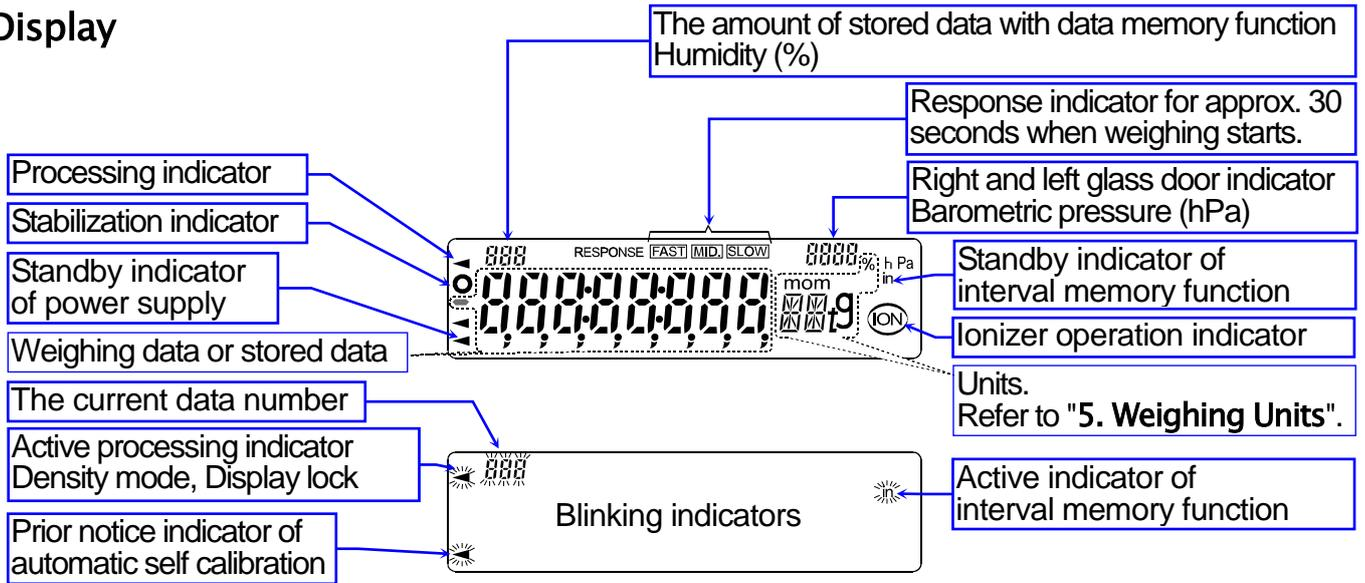
The interval memory function is used to store the weighing data periodically. Refer to "12. Data Memory".
